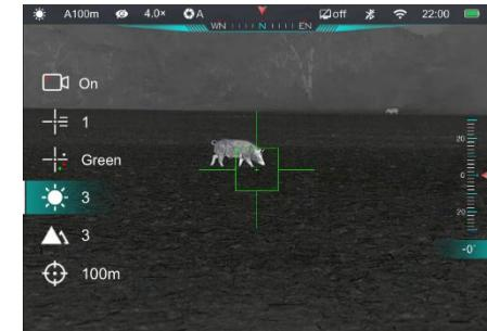
video recording option, and press the **Controller (4)** to turn the video recording function on/off.
