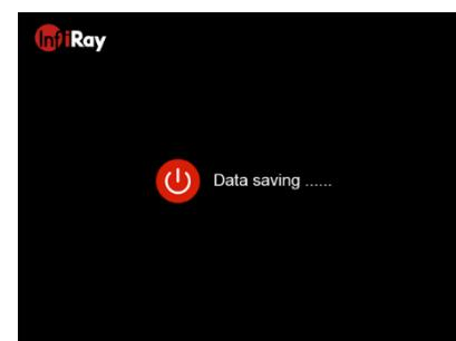
prompt interface is displayed. When the data is saved, the display turns black and the device is off. **When the device is powering off and saving data, do not disconnect it from its power source. Otherwise, the data cannot be saved.**
