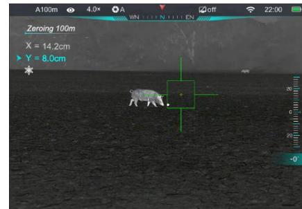
reticle) do not match, keep the aiming position still, and meanwhile, press and hold the **Controller (4) + Power button (5)** at the same time until a snow-like freezing icon
